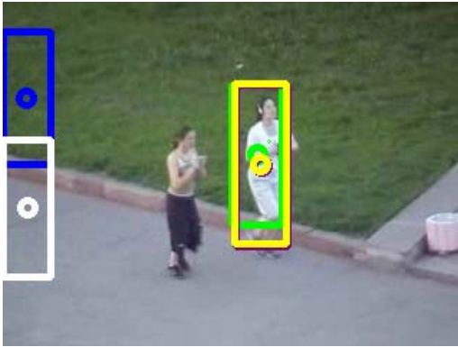
Fig. 6: Scenario illustrating the case when only the two worst-performing trackers in the ensembles are correct, whereas the generally superior TLD and ST fail. The blue, green, white and purple boxes correspond to the outputs of TLD, CMT, ST and GT, respectively. The yellow box is the output of the fused approach. Best viewed in color.
